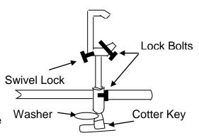
2. Attach the clip end of the safety cable around the truss from the handle of the Hurricane and attach the cable to itself. You may now adjust the position of the Hurricane II<sup>TM</sup> with the wrench, spinning or tilting as desired. Do not loosen any of the anchor bolts for movement without the safety cable attached first.
